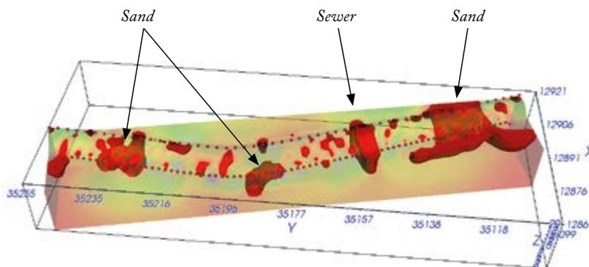
*3D resistivity model of an embankment. The granular sediment bodies are highlighted.*
